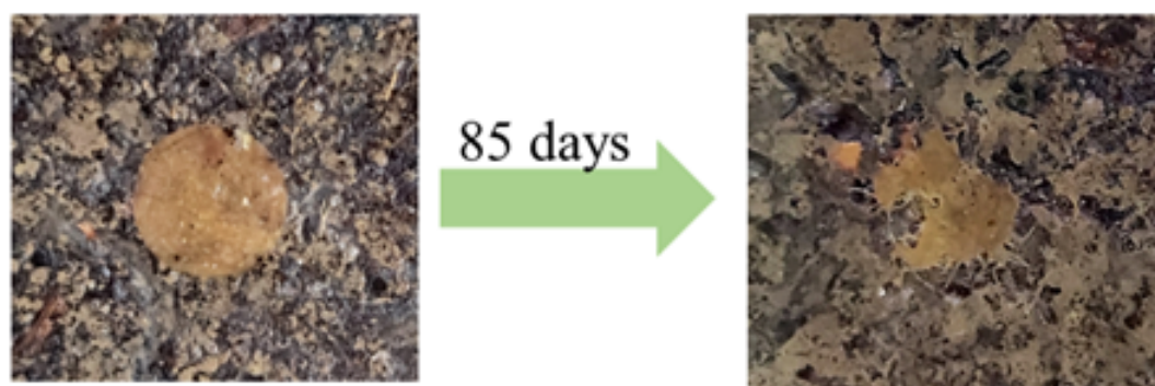
Figure 4. Biodegradability test of cHM before and after 85 days.
