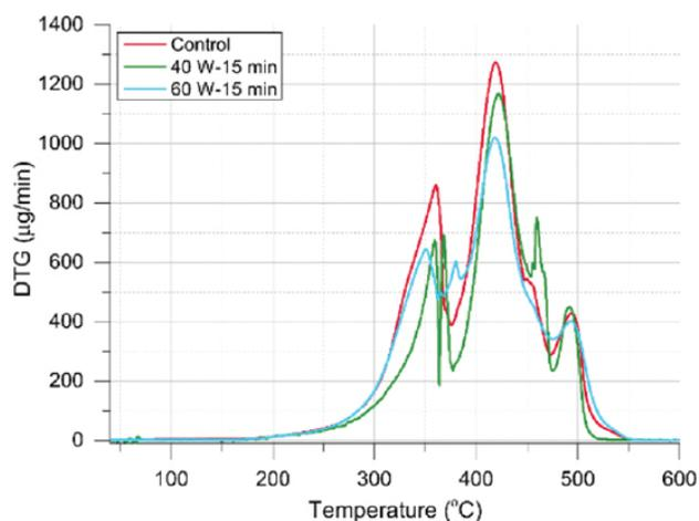
**Figure 5.** Differential thermogravimetric plot of the oils
