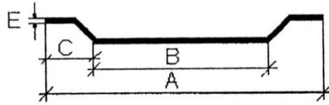
Figure 2. The shape of fibers used as fiber-reinforcement
