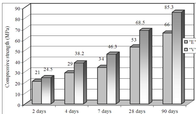
Figure 5. Comparative review of compressive strength on both series 'E' and 'V'
