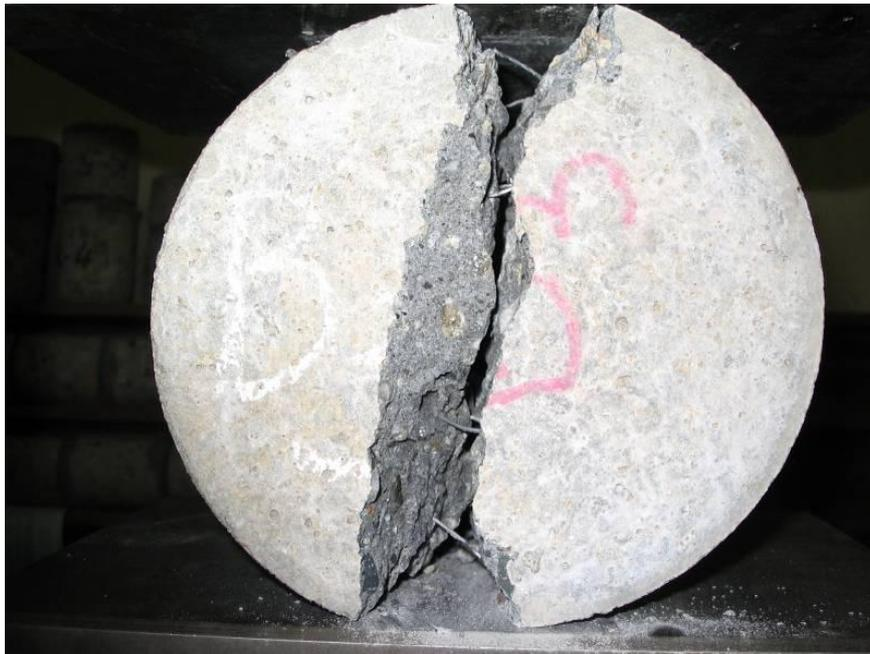
*Figure 6 . Splitting tensile test - Steel fibers continue to bridge the crack after the breakage of the specimen*
