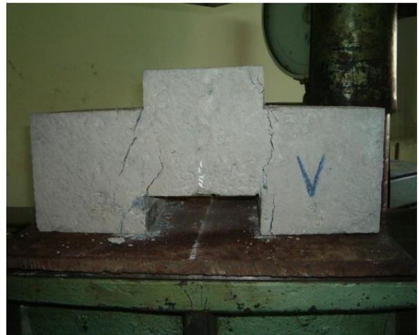
*Figure 7. Shear strength test*
