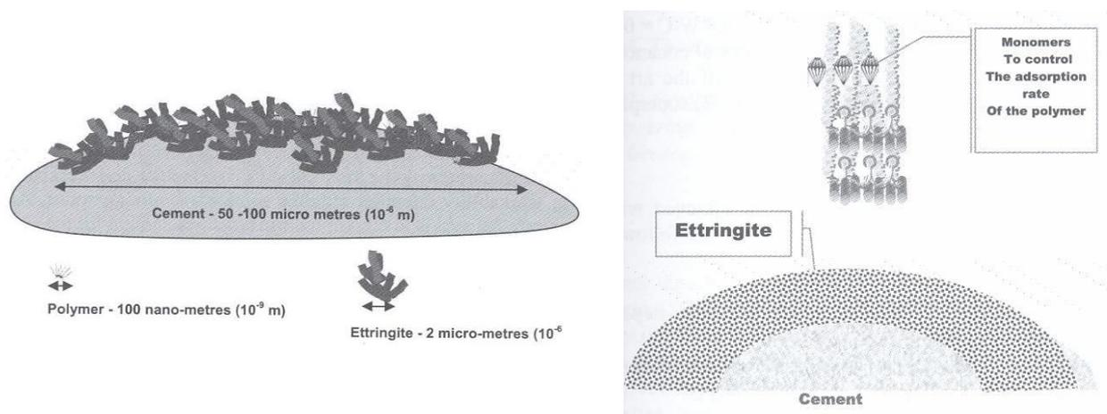
Figure 1. a) Mechanism of action of superplasticizer and b) The "parashoot" effect of monomeric superplasticizer
