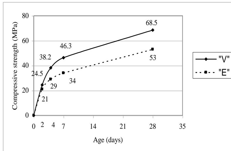
Figure 4. Compressive strength growth in time
