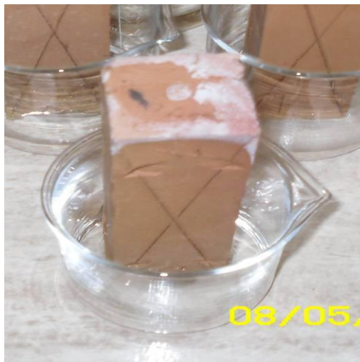
Figure 4. The efflorescence white deposits occurred on fired prisms made with clay without ameliorative additive
